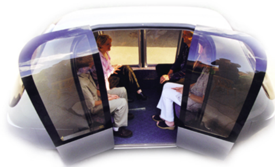
Figure A-15 - ULTra Door Opening
