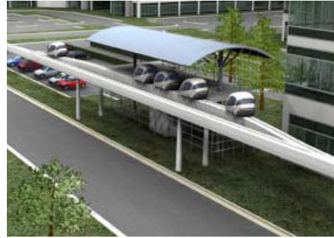
Figure A-18 - Off-line Station
